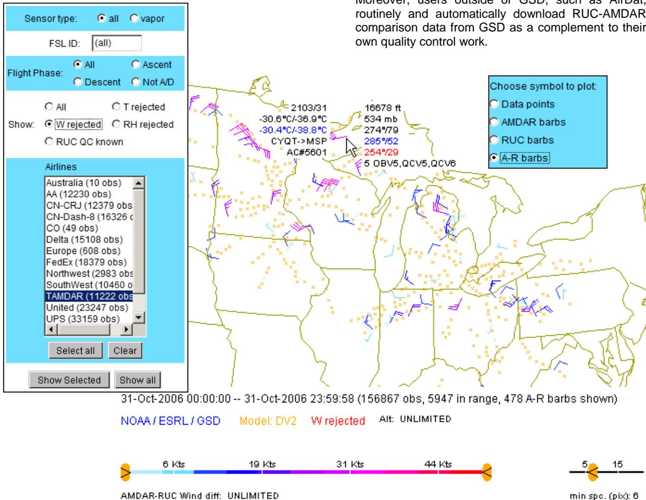
Figure 3. Plan view of AMDAR and RUC values from [http://amdar.noaa.gov/ruc\\_acars/plan\\_view/](http://amdar.noaa.gov/ruc_acars/plan_view/), showing plan-view map and 'select' window. This plot shows vector difference between TAMDAR and dev2 winds.
