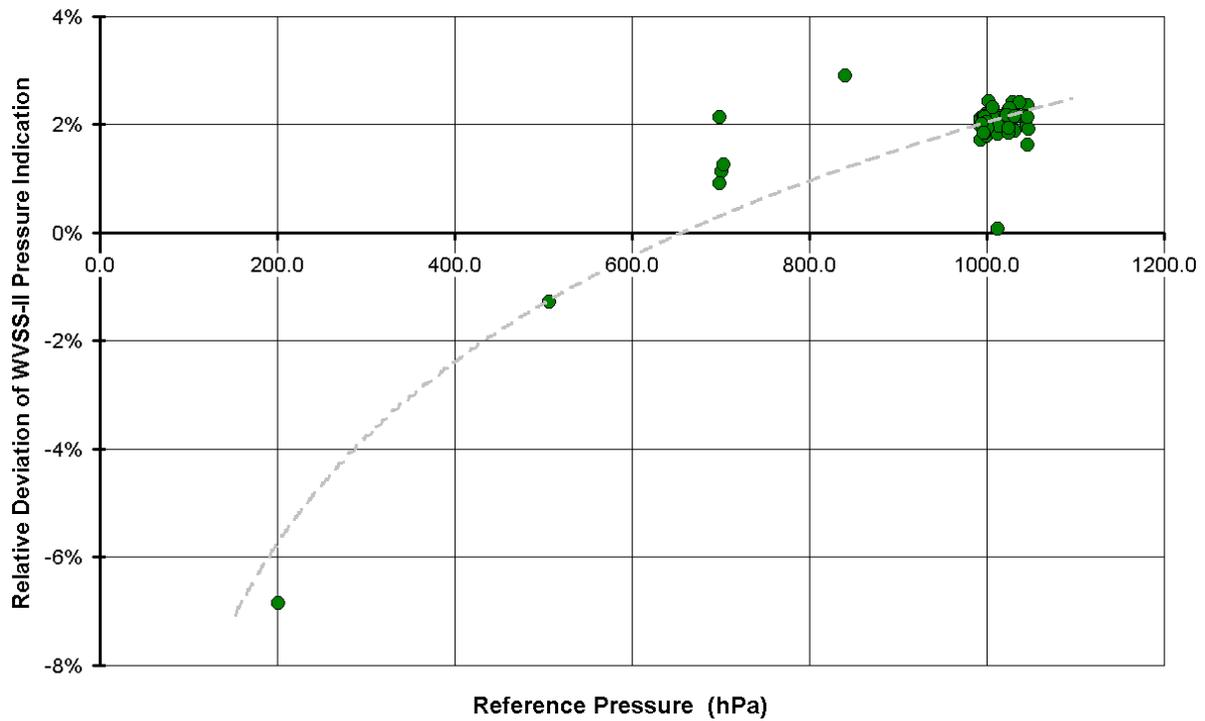
Fig. 7: The relative deviation of the WVSS-II's pressure readings against the climate chamber's measurements.
