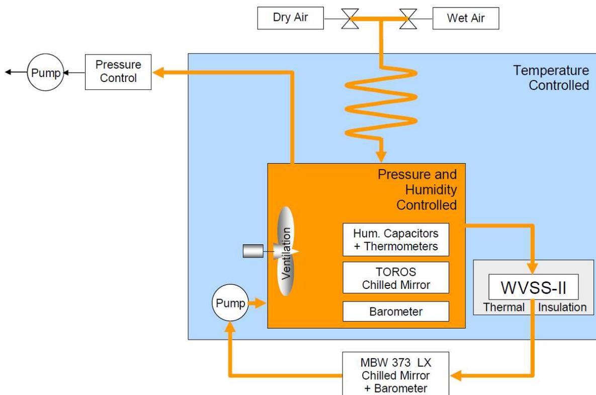
Fig. 2: Block diagram of the DWD climate chamber at the Meteorological Observatory Lindenberg, Germany.
