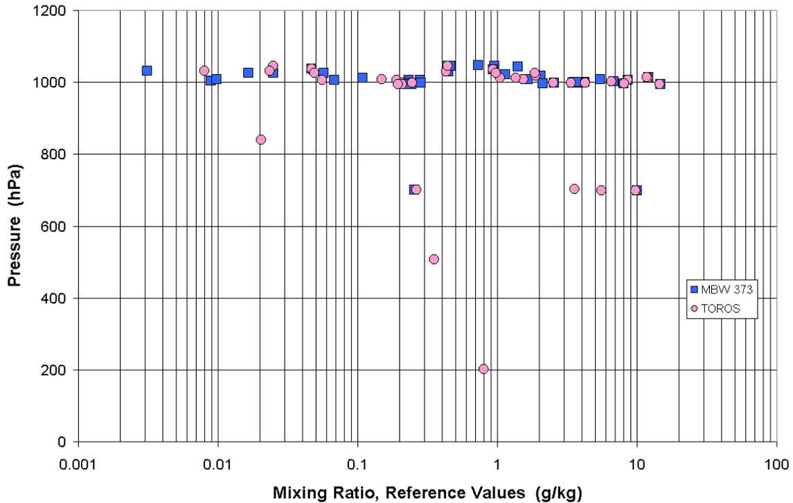
Fig. 5: Water vapour reference measurements as function of mixing ratio and pressure level. Data for the two different reference sensors MBW 373 and TOROS are shown separately.
