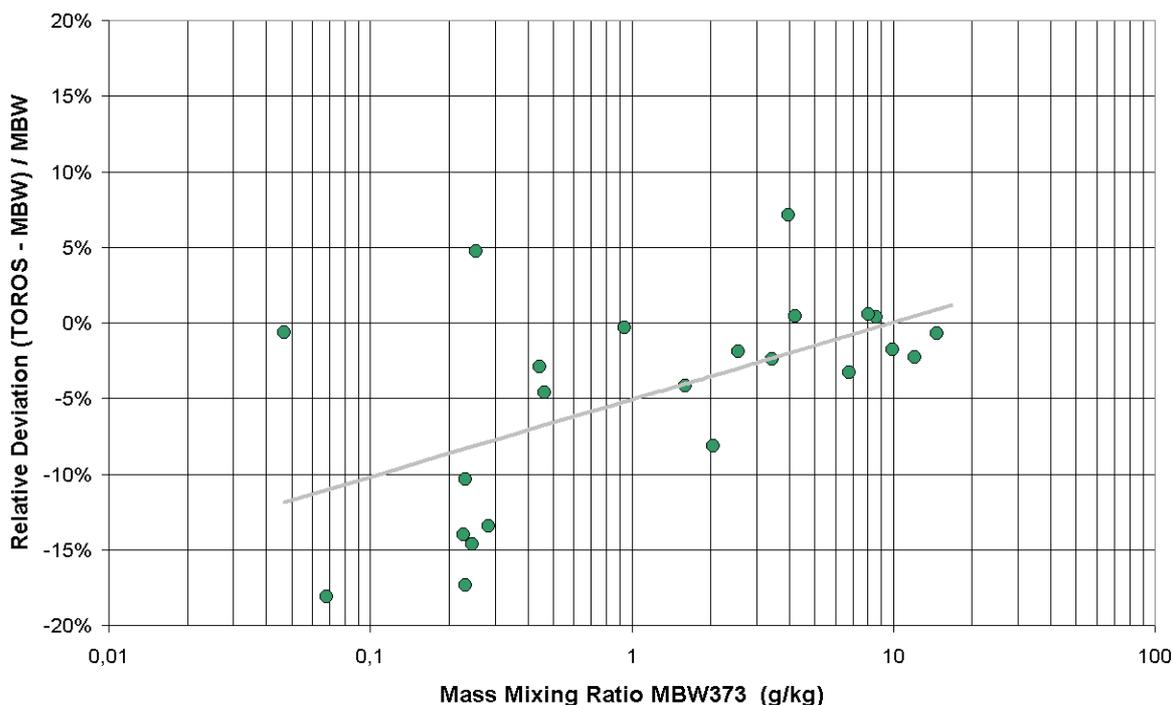
Fig. 4: Relative deviation between the reference sensors MBW 373 and TOROS.
