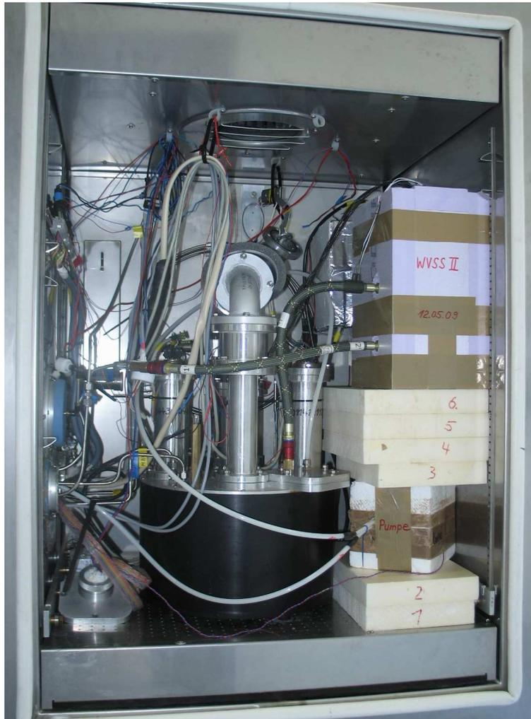
Fig. 3: View into the climate chamber's temperature controlled bin. The black vessel in the middle is the humidity and pressure controlled bin.
