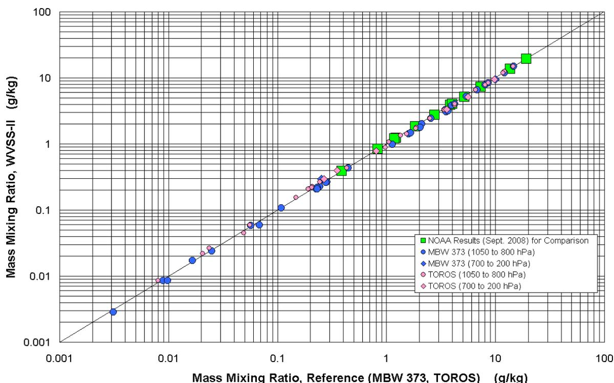
Fig. 8: The WVSS-II's mixing ratio readings plotted in a log-log diagram against the climate chamber's reference measurements. The differently marked data points distinguish
