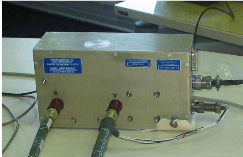
Fig. 1: The System Electronics Box (SEB) of the aircraft humidity sensor type WVSS-II, Version 3 (2009).
