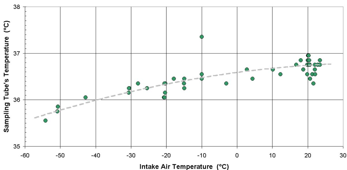
Fig. 6: The air temperature inside of the sampling tube versus the intake air temperature at a flow rate of 1 l/min.
